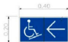
Sign indicating for wheelchair form corridor to the ramp 1 and 2 higher than the floor 1.50 m.
